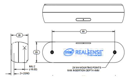
Figure 1: Rear of the Intel RealSense Depth Camera D455. All units in millimeters. Taken from [?].
